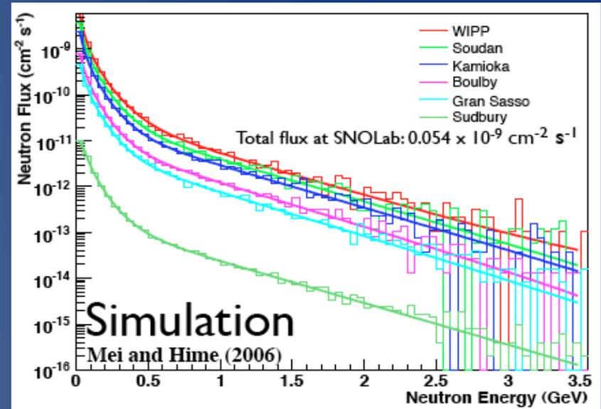
A conservative estimate of muon induced neutrons that originate in the cavern walls with no tagged muon and then create a background signal in the ROI is  $<0.1$  / year
