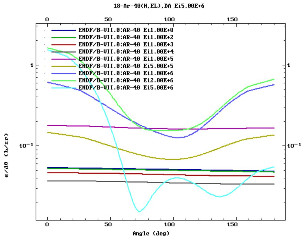
Geant4 simulations of monoenergetic neutrons elastically scattering in Argon
