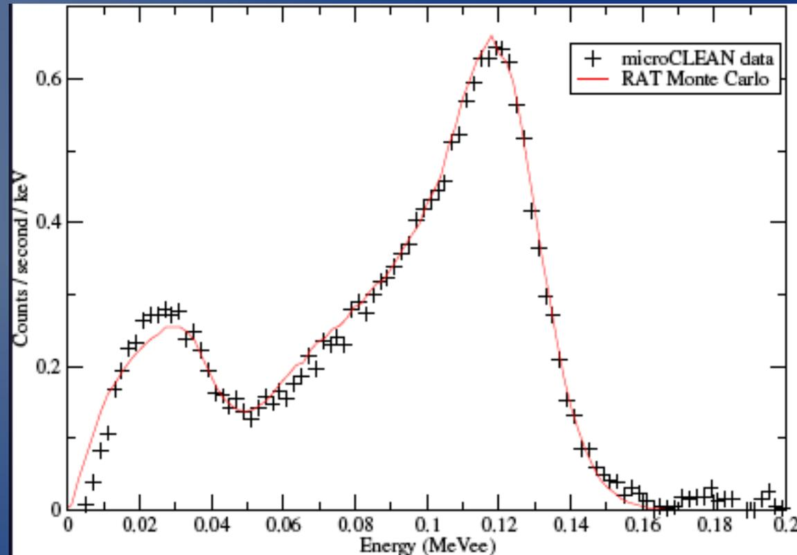
MicroCLEAN comparison of data and simulation Of  $^{57}\text{Co}$  gamma rays
