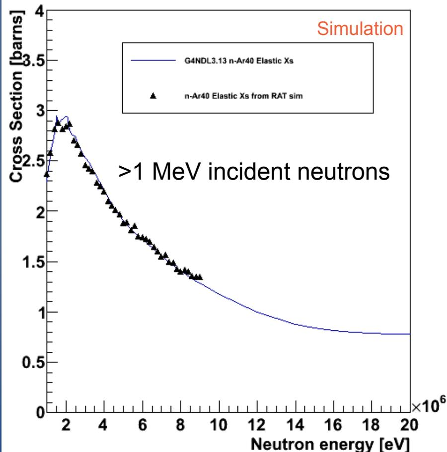
Monoenergetic neutrons shot into liquid natural argon, Inelastic processes turned off
