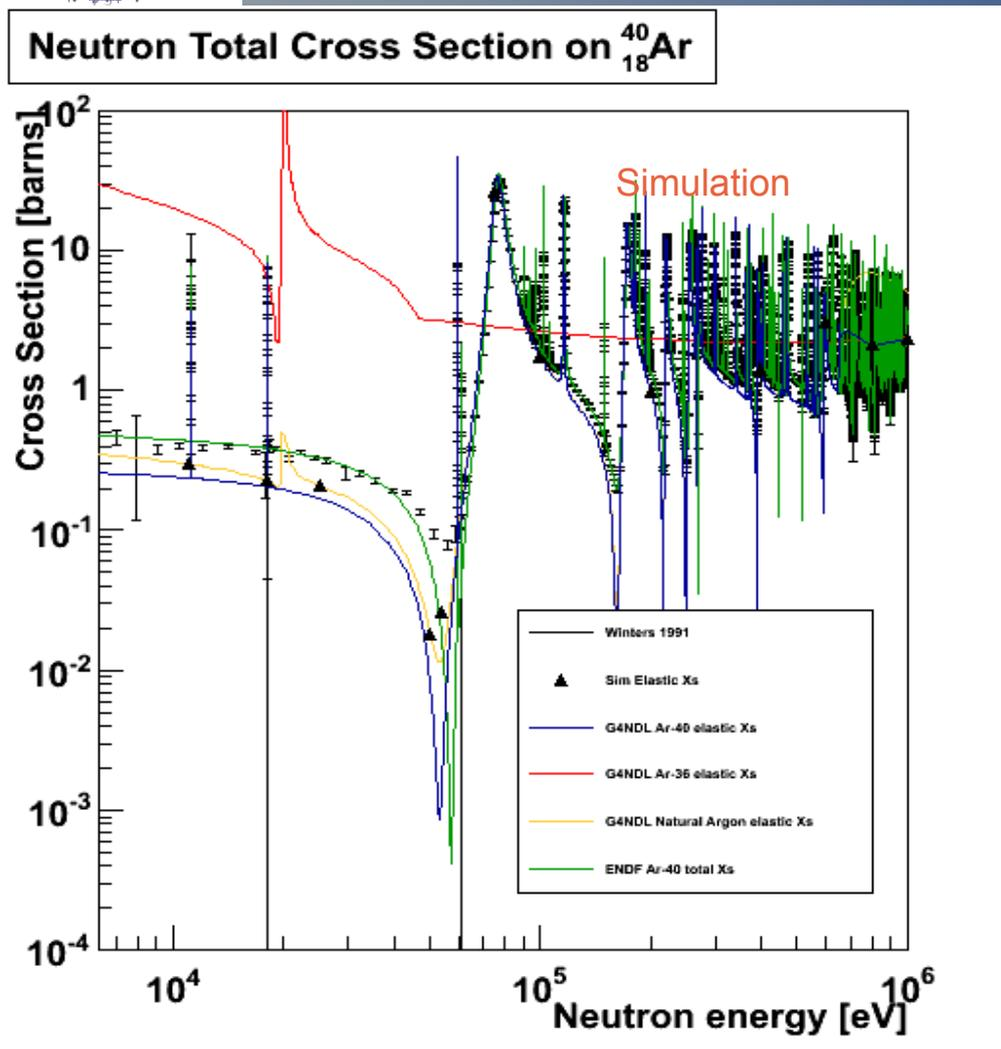
Measurements and simulations have really been done with natural argon, at low energies  $^{36}\text{Ar}$  becomes important!
