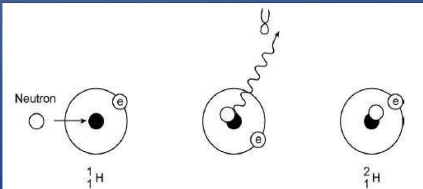
Neutron Capture: Cross section dominates at thermal energies (0.025 eV) also resonances at keV energies
